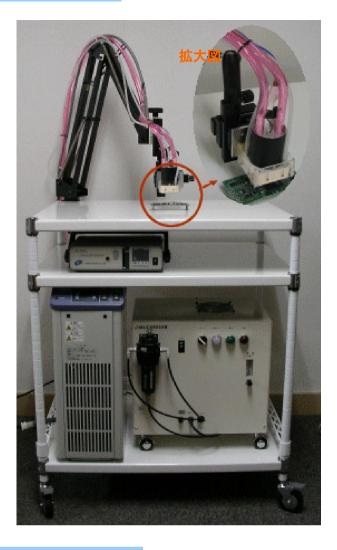
It is a system got using the top-plat of a Wagon as an experiment plate. Since other Articulated arms are equipped with the TempTest Head it is not installation position of an Experiment subject. Moreover, the soft contact To a subject is possible by adopting a precision Movable stage at the tip of an arm. By carrying all the peripheral equipment in a Wagon, the minimum occupancy area is realized And movement of convenience improves also in A required environment.
